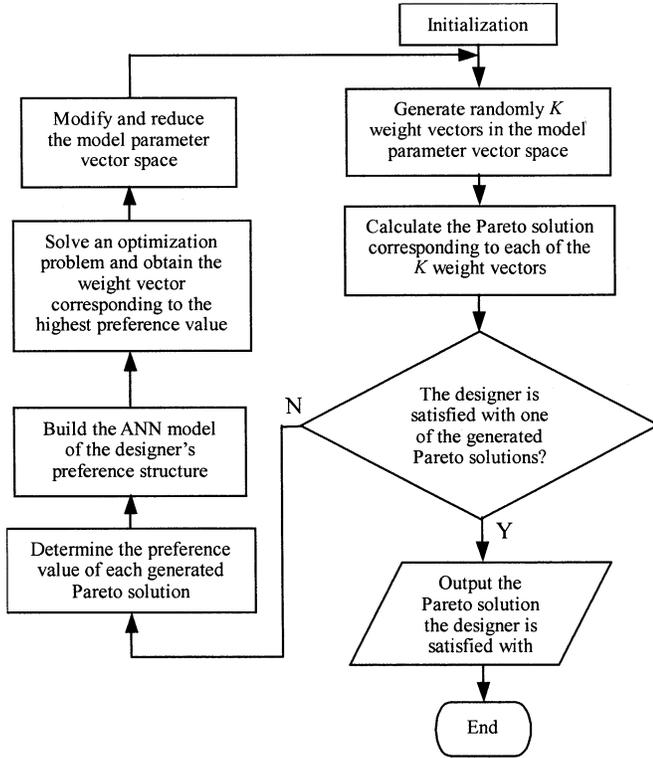
Fig. 3. The flowchart of the IIMOM procedure.
