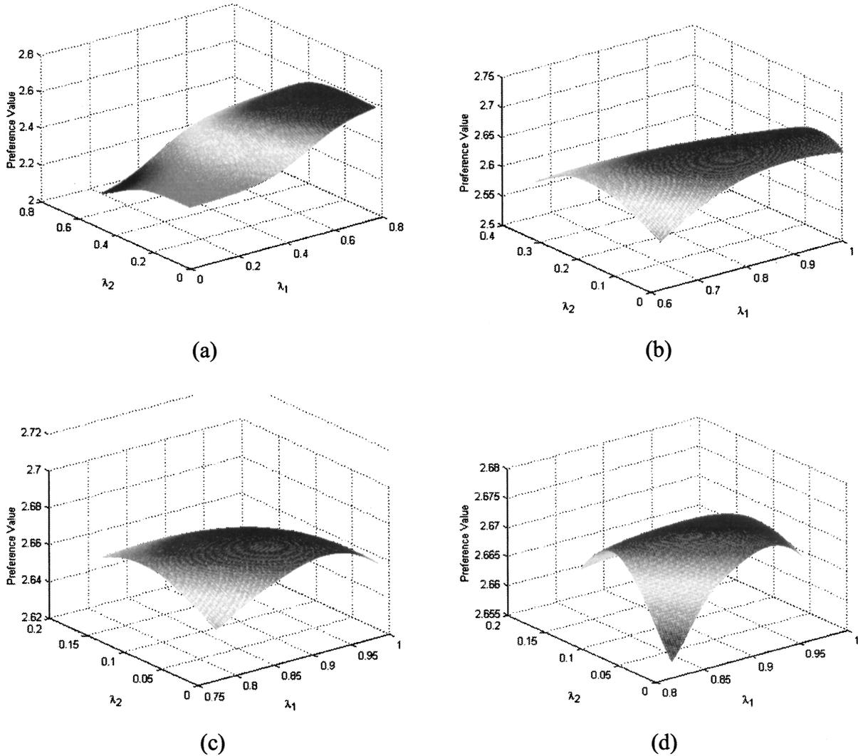
**Fig. 4.** The ANN model of the designer's preference structure in the case of the linear value function: (a) at the second iteration; (b) at the fifth iteration; (c) at the eighth iteration; and (d) at the 10th iteration.
