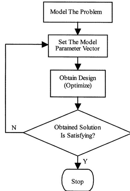
Fig. 1. The general multiobjective optimization procedure.
