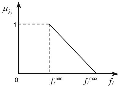
Fig. 2 Linear satisfaction degree function for *i*th objective
