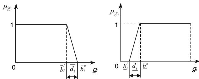
Fig. 3 Two linear sufficiency degree functions for constraints
