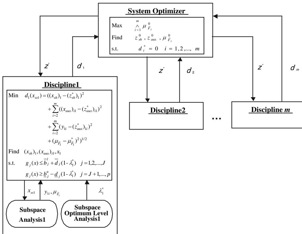
Fig. 6 The architecture for the FSSDCO using  $\alpha$ -cuts method
