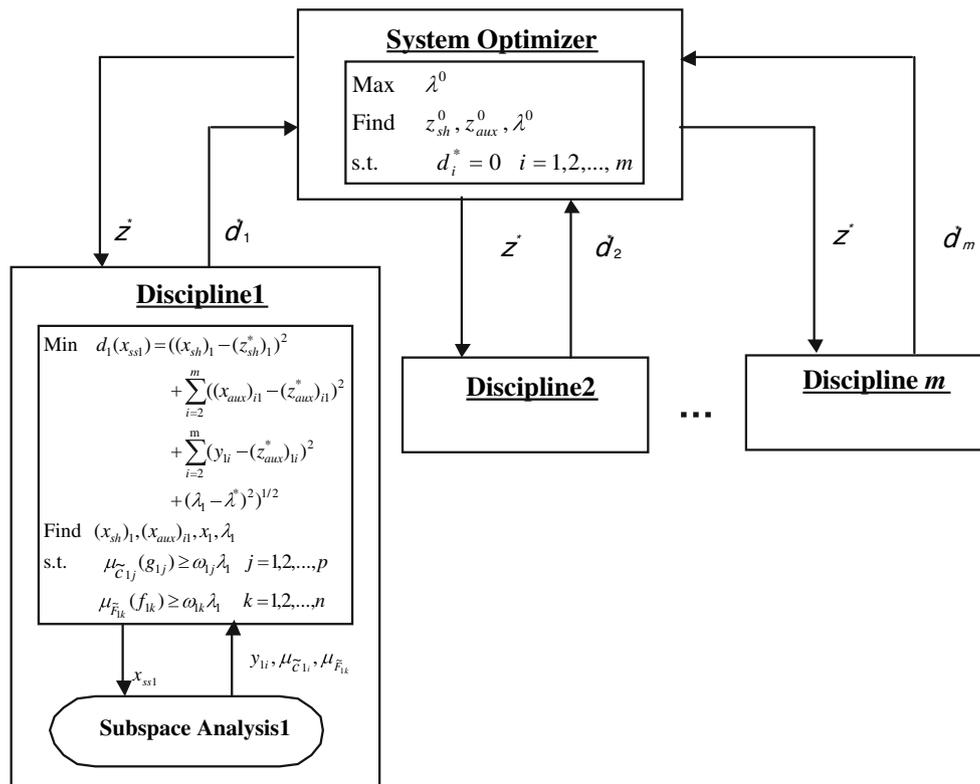
Fig. 4 The architecture for FSSDCO based on weighted Max–Min method
