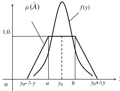
Figure 1. The membership function of  $\tilde{A}$  and the distributing density function of  $y$ .
