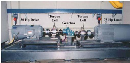
Fig. 4. Mechanical diagnostic test bed.
