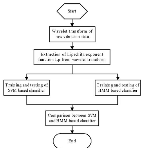
Fig. 1. The diagram of condition monitoring system.
