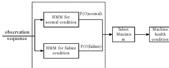
Fig. 7. Structure of HMM based classification system.
