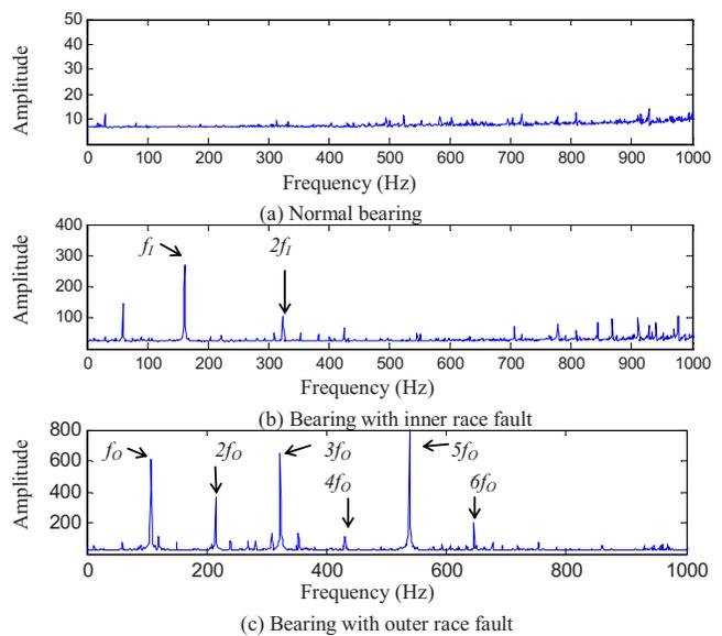
FIG. 6. (Color online) Identification of fault-related characteristic components under motor speed 1797 rpm and load HP 0.
