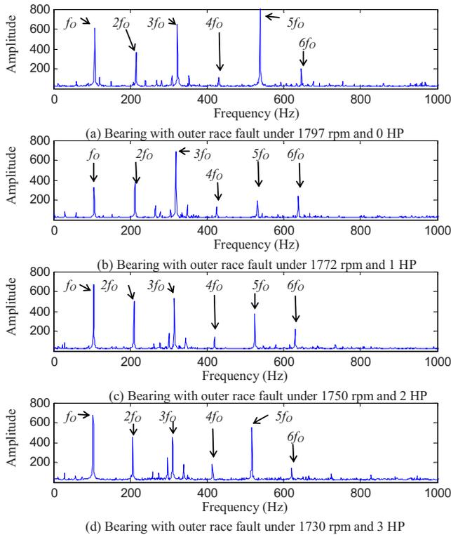
FIG. 7. (Color online) Identification of characteristic components of bearing with outer race fault under different speeds and loads.
