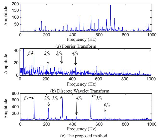
FIG. 9. (Color online) Comparison of characteristic component identification using vibration of bearing with outer race fault.
