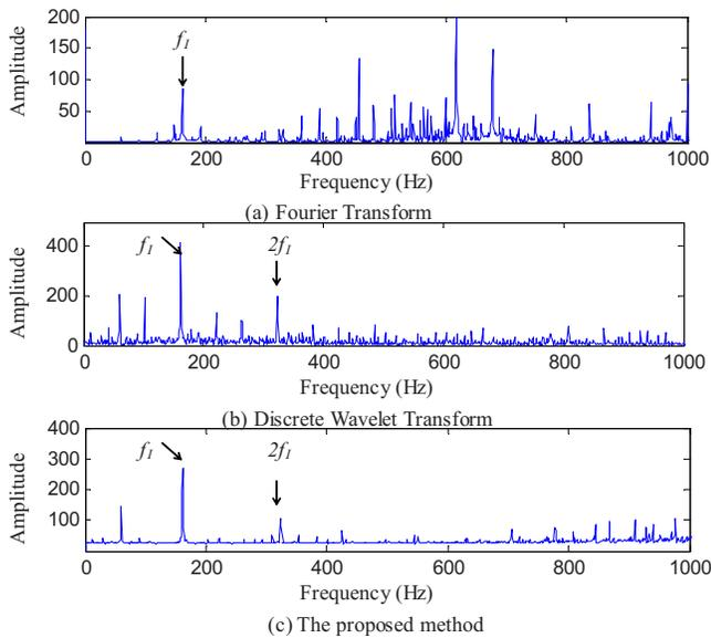
FIG. 10. (Color online) Comparison of characteristic component identification using vibration of bearing with inner race fault.
