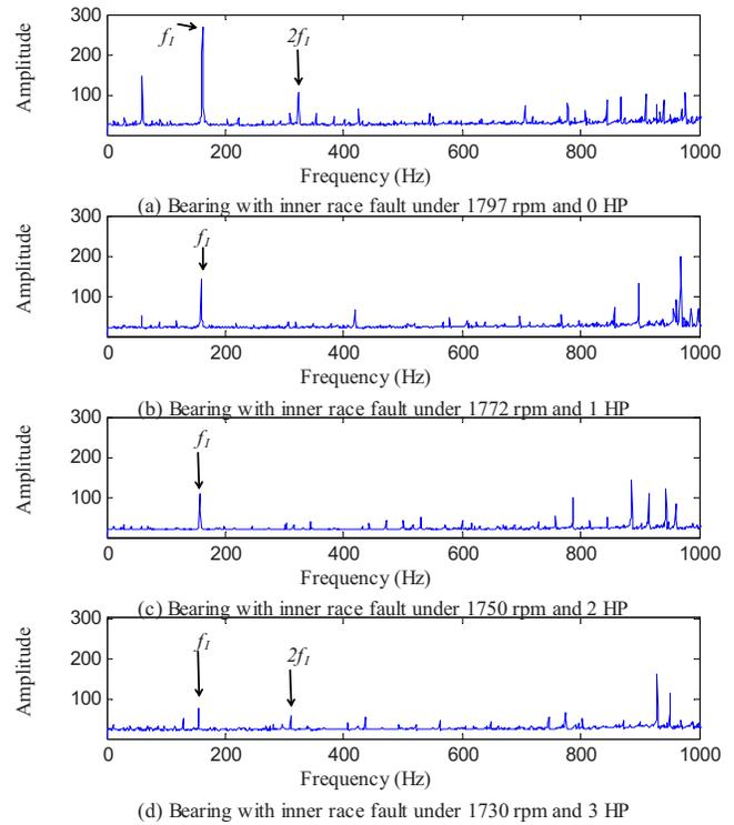
FIG. 8. (Color online) Identification of characteristic component of bearing with inner race fault under different speeds and loads.
