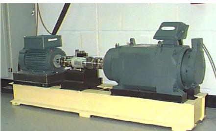
FIG. 2. (Color online) Test rig of bearings.
