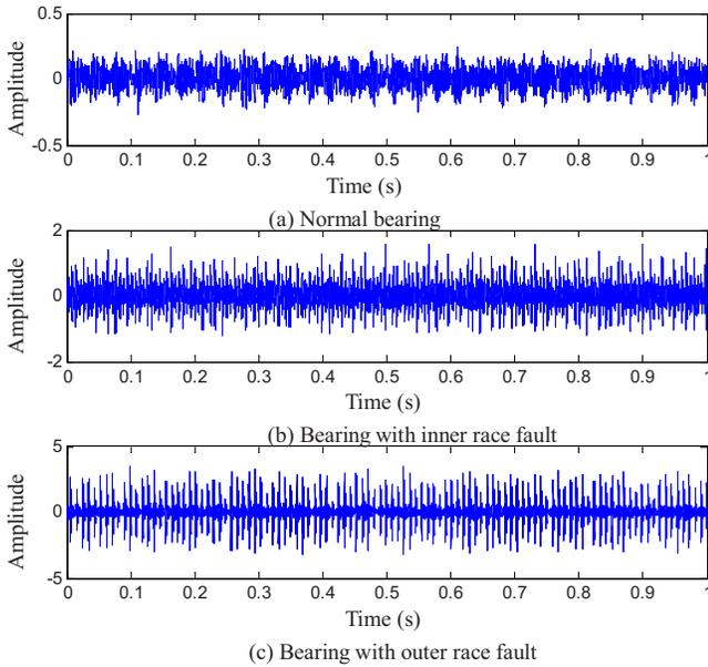
FIG. 3. (Color online) The original signals under motor speed 1797 rpm and load HP 0.
