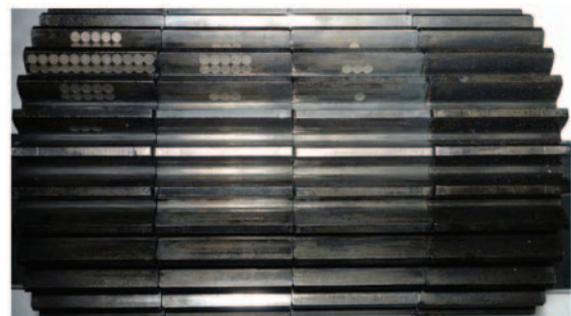
Fig. 10 Planet gears with artificially created pitting damage (from left to right corresponding to the damage degrees of severe, moderate, slight, and baseline)
