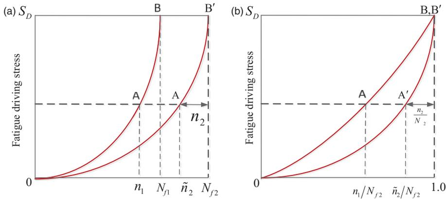
Figure 2. Non-linear damage accumulation (high-to-low load sequence). (a)  $N_f$ , cycles and (b)  $\frac{n_i}{N_f}$ , cycle fraction.
