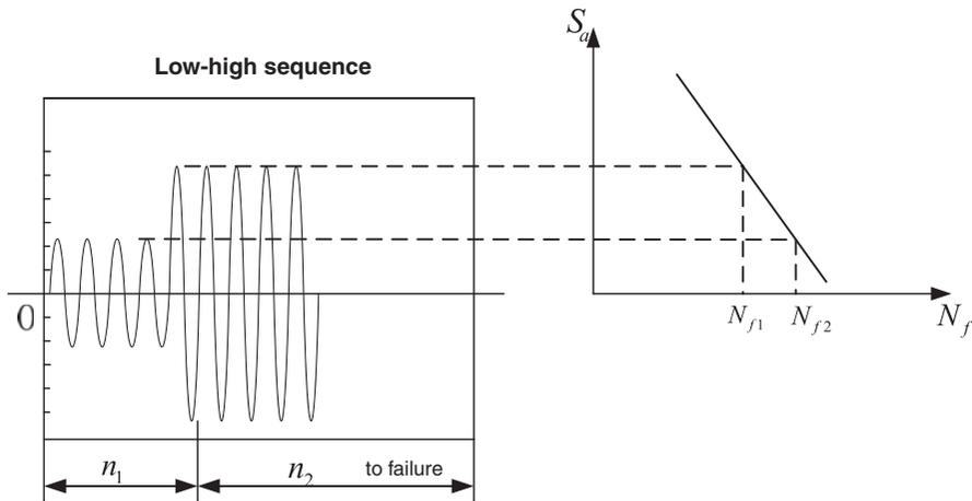
Figure 3. A two-step block loading under low-to-high load sequence.
