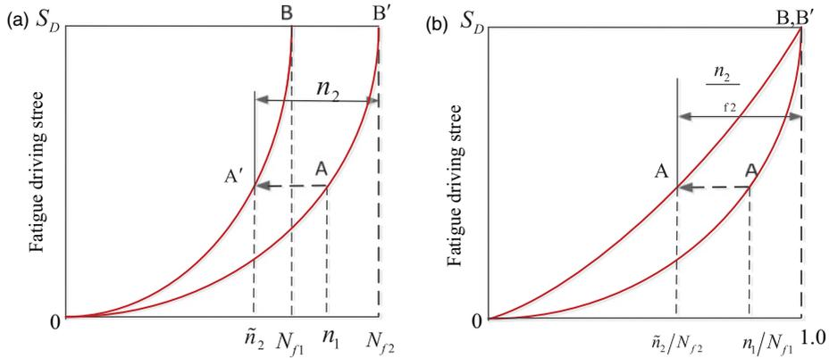
**Figure 4.** Non-linear damage accumulation (low-to-high load sequence). (a)  $N_f$ , cycles and (b)  $\frac{n}{N_f}$ , cycle fraction.
