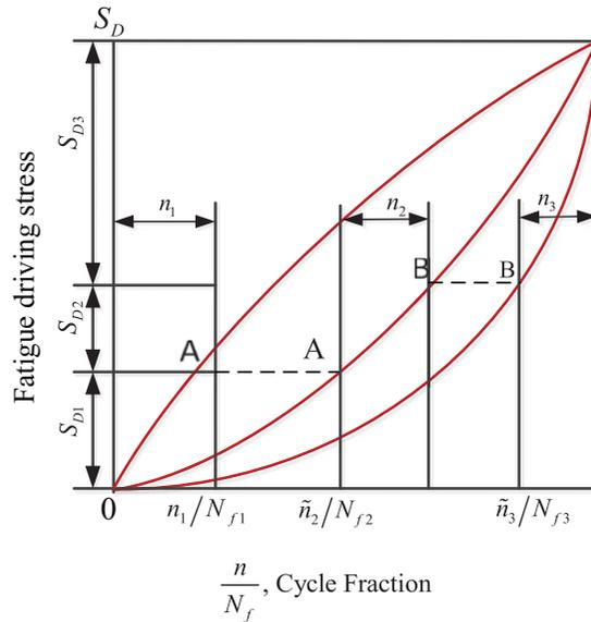
**Figure 5.** A block of three-level fatigue loading.
