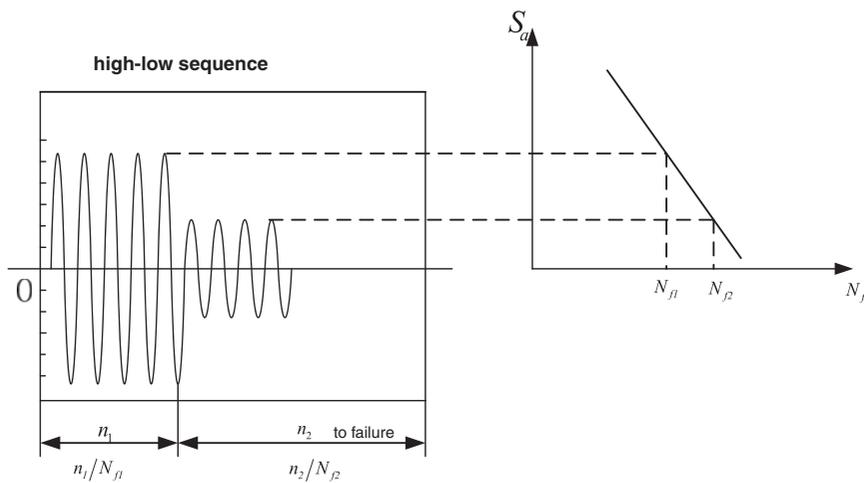
**Figure 1.** A block of two-step high-low sequence loading.
