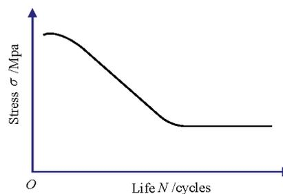
Figure 1. Schematic interpretation of  $S-N$  Curve.
