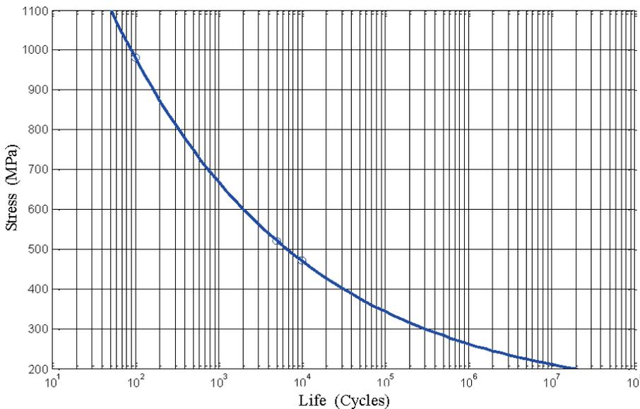
**Figure 3.** Working  $S-N$  curve of an aircraft engine.
