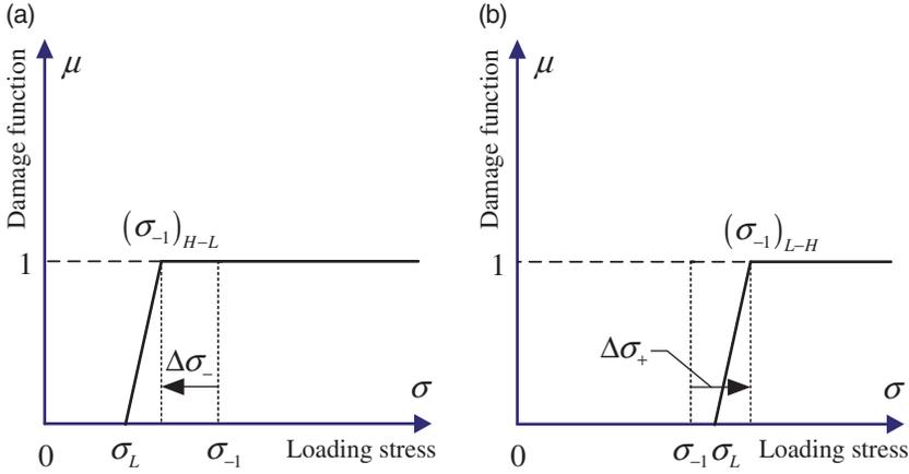
**Figure 4.** the proposed Miner rule under low amplitude loading strengthening and different load sequences (using increasing half-trapezoidal shaped MFs).
