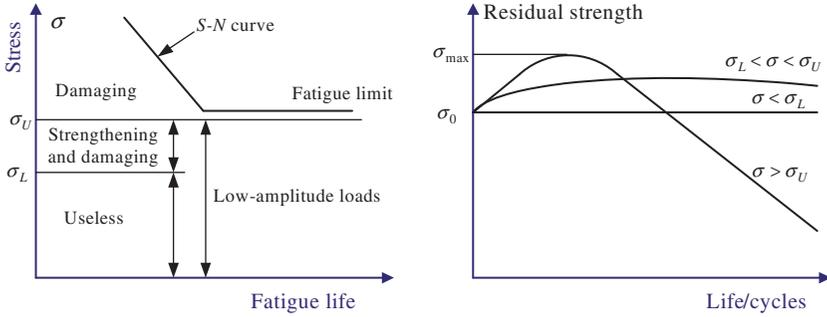
Figure 1. Load region, its strengthening and damaging in different cycle ratios.
