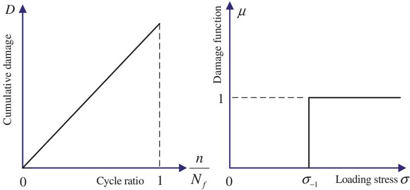
Figure 2. Miner rule and its damage function.
