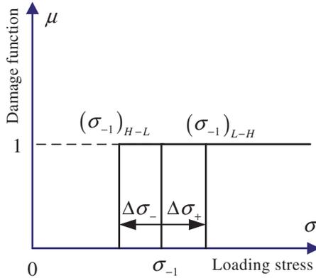
Figure 3. The change of fatigue limit under different loading sequences.
