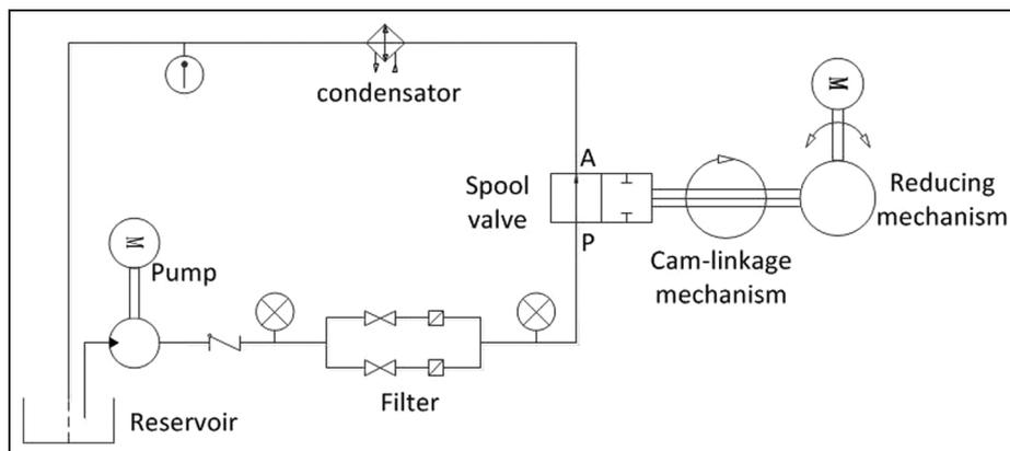
Figure 5. Basic diagram of wear experiment for a DDV.
