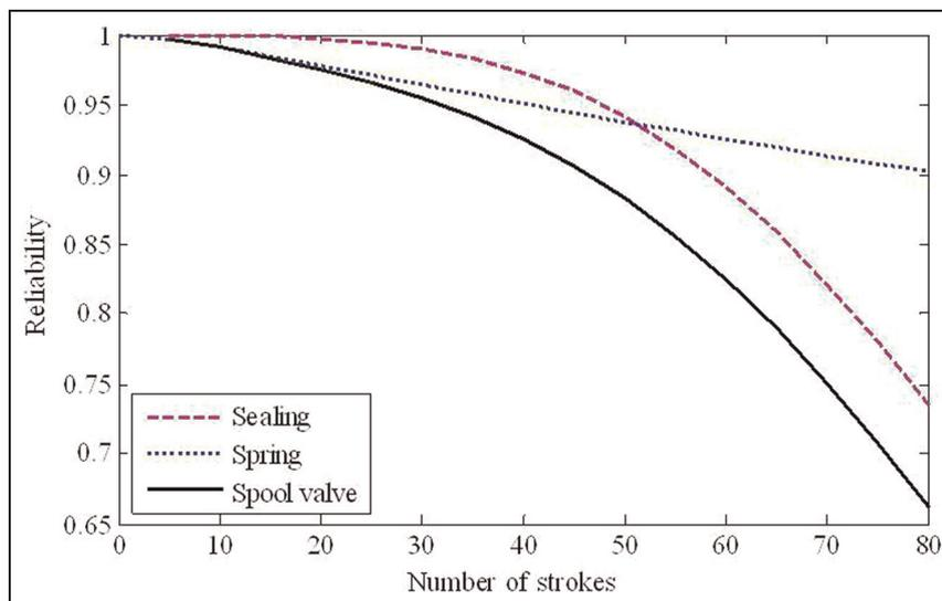
**Figure 7.** Reliability estimation of the sealing, the spring and the spool valve.
