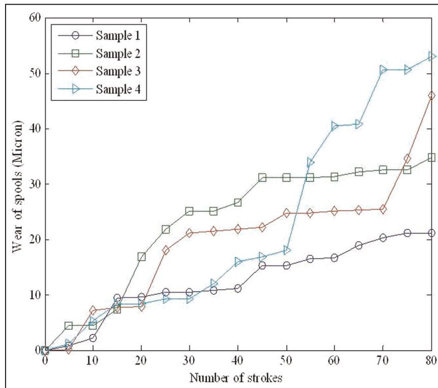
**Figure 6.** Wear degradation paths of spools.
