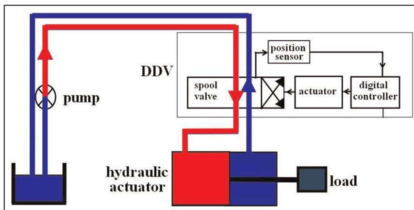
**Figure 1.** Hydraulic circuit of a DDV with pump supply and load. DDV: direct drive electrohydraulic servo valve.
