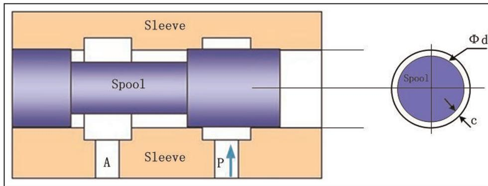
Figure 4. Schema of the spool valve and clearance.
