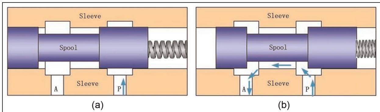
**Figure 3.** Configurations of the spool valve in (a) closed position and (b) open position.
