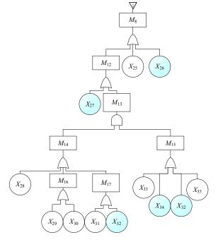
Fig. 5. The fault tree of "manual intervention fail"
