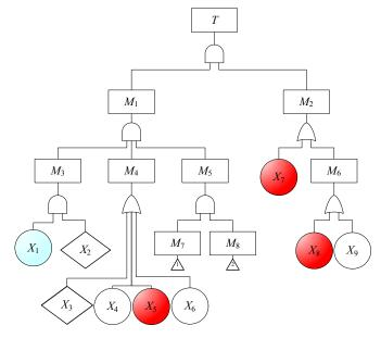
Fig. 3. The fault tree of train rear-end collision accident
