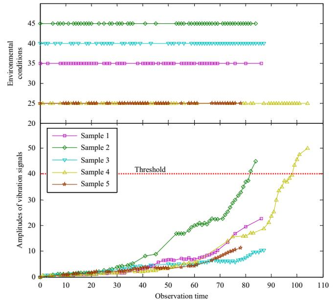
Fig. 2. Environmental conditions and amplitudes of vibration signals for DL150 CNC heavy duty lathes.
