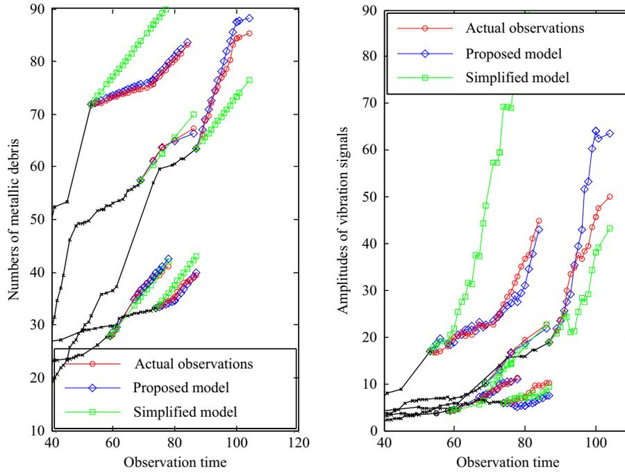
Fig. 7. Comparison of degradation predictions of the proposed model and the simplified model.
