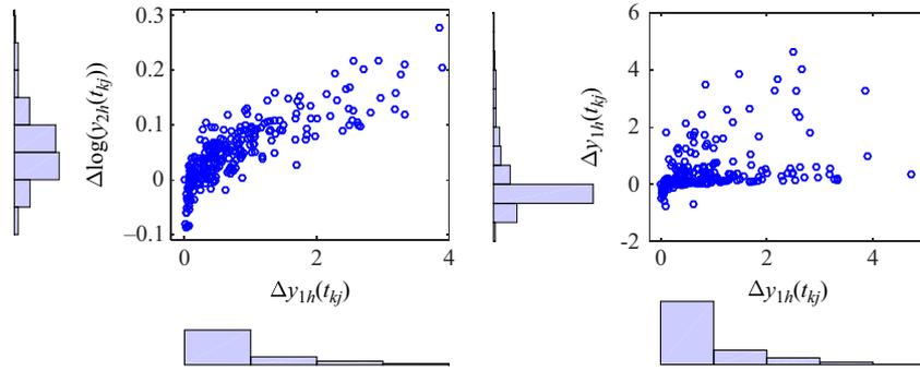
Fig. 3. Scatter plots of degradation increments of the number of metallic debris and the nominal (logarithmic) amplitudes of vibration signals.
