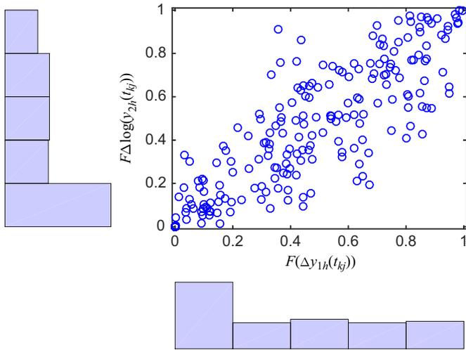
Fig. 4. Scatter plots of CDFs of degradation increments of the number of metallic debris and the logarithmic amplitudes of vibration signals.
