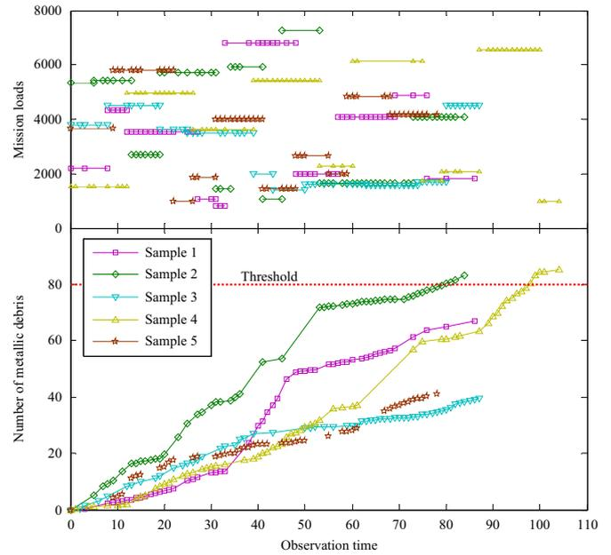
Fig. 1. Mission loads and number of metallic debris observed for DL150 CNC heavy duty lathes.
