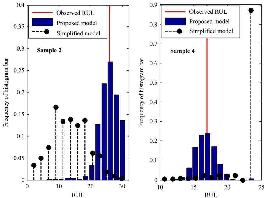
Fig. 8. Comparison of RUL assessment of the proposed model and the simplified model.
