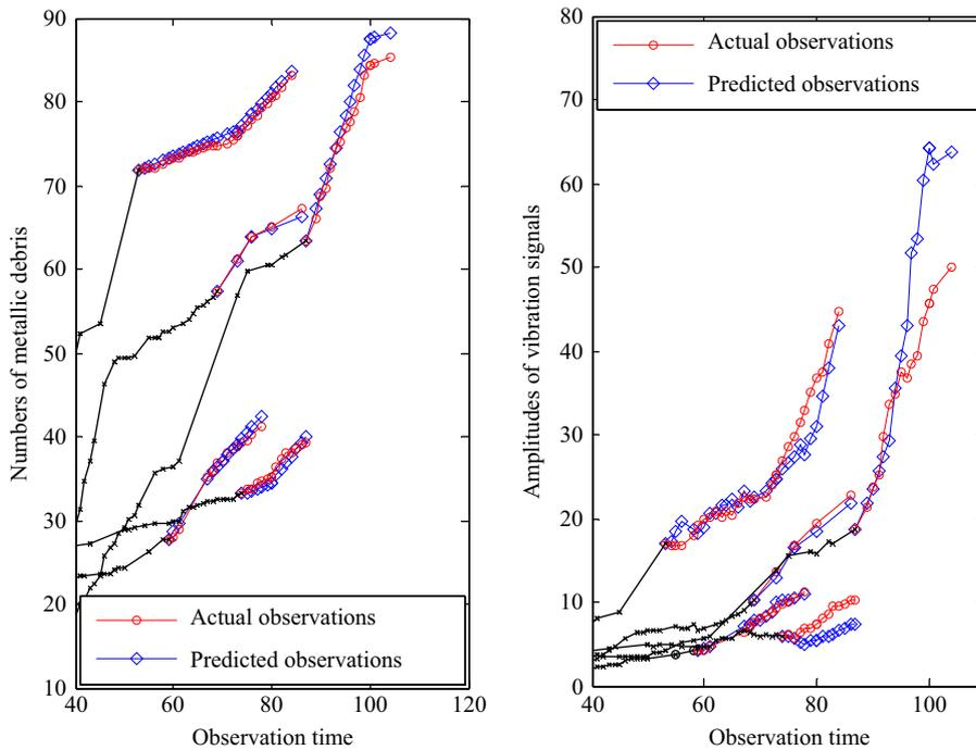
Fig. 5. The predicted vs. the actual degradation observations for the latest two missions.
